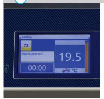
Mix cooling and ageing are performed in a dedicated cooling vat provided with an improved cooling system with a 9-speed inverter for a quick mix cooling up to +4°C and subsequent ageing. This prevents mix stressing and the risk of impairing the benefits of homogenization.
