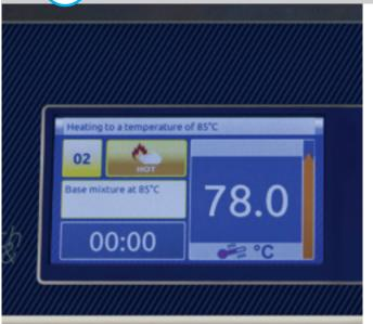
Heating at 85°C and then pre-cooling at 72°C as required to sanitize the bacterial load and activate the hydrocolloid ingredients of the mix. Genius combines the characteristics of the well-known and appreciated Sweety pasteurizer of TTi series with an improved resistance heating system up to 98 °C to reduce processing times.
