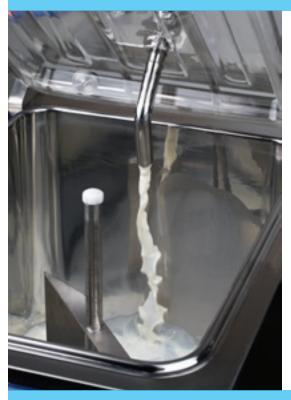
Rubber pipes are standard supplied, stainless steel pipes are supplied as optional. They are provided with special fittings to pour mix under pressure in total safety and without the risk of accidental leakage.
